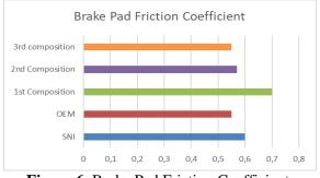
Figure 6. Brake Pad Friction Coefficient Comparison
