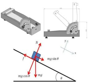
Figure 4. Friction Coefficient Tester
