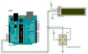
Figure 1. Temperature sensing wiring diagram
