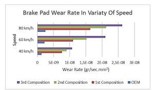
Figure 7. Brake Pad Wear Rate Comparison
