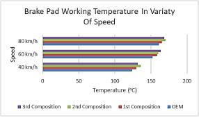
Figure 8. Brake Pad Working Temperature Comparison
